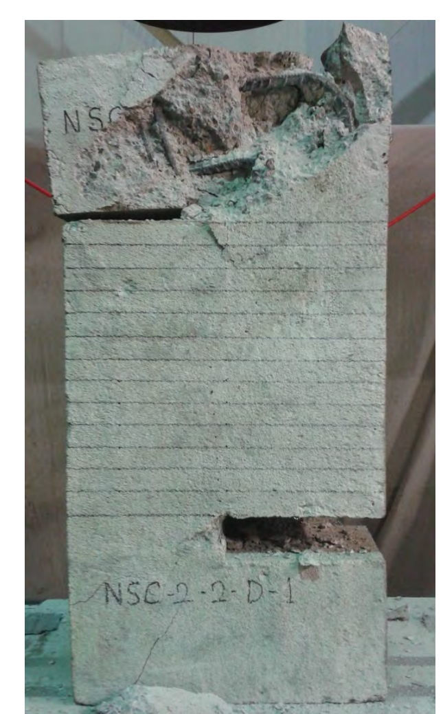
NCS with 1.6% reinforcement
