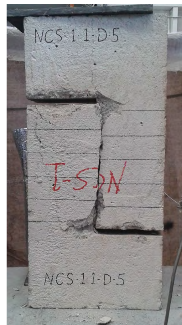
NCS with 0.8% shear reinforcement
