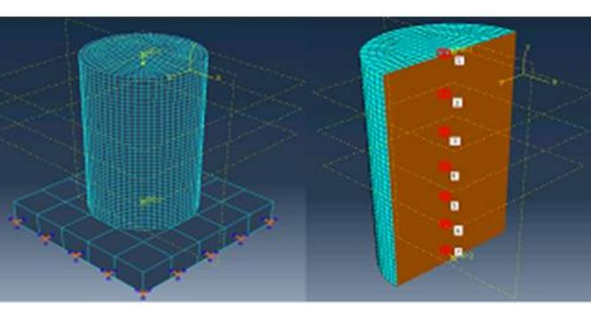
FEM model of the drop-hammer test
