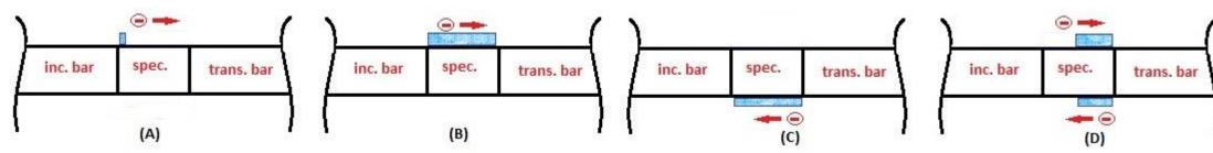
(A) "wave 1<sup>st</sup> face" - the stress wave reach the first face of the specimen. (B) "Wave 2<sup>nd</sup> face" - the stress wave reach the second face of the specimen. (C) "Reflected wave 1<sup>st</sup> face" – the reflected wave from the 2<sup>nd</sup> face reach the first face. (D) between time marks (B) and (C) - the reflected wave from the 2<sup>nd</sup> face reach the specimen's midspan (not marked on charts).
