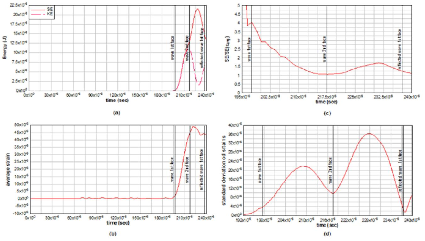
strain energy was defined by using the theory of elastic waves. It was shown that part of the kinetic energy remained in the specimens, and the stress distribution along the specimen was not uniform. Finally, a short comparison of the SHPB and the drop-hammer test were presented.
