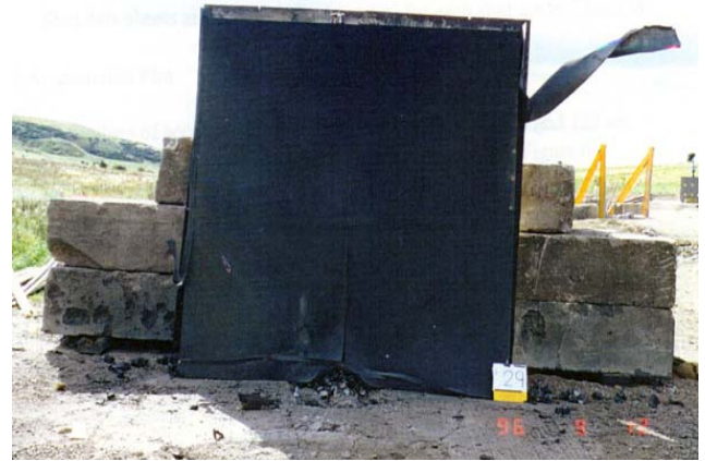
View after three explosive tests using : 30 kg PE4 AT 3.85 m, 15 kg PE4 AT 0.9 m.
